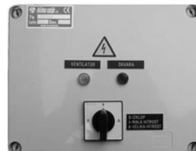
The switchbox is designed for ON/OFF and lower or higher RPM selection, including electromotor thermal protection for roof fans SVH2 and SVV2 sizes 400/315 to 560/500. The motors are factory  $\Delta$  connected, therefore bridge connectors have to be removed from the fan terminal box.
