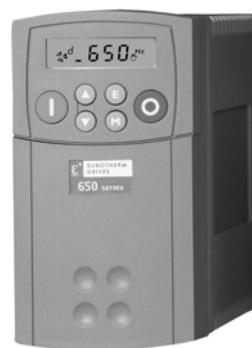
One phase frequency converters are used for RPM regulation of three phase electromotors connected  $\Delta$ 3x230V with power up to 1,5 kW. They enable optimal control and protection of el. motors. They can regulate two or more fans parallel as long as the current limit is not exceeded. They also have TK contacts with no automatic restart.
