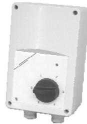
The five-stage voltage regulator allows starting/stopping and manual setting of five speeds for the fans SVH2 and SVV2 sizes 250/200 and 315/250. It can regulate two or more fans parallel as long as the current limit is not exceeded. It can be used only with motors with built-in overheating protection.
